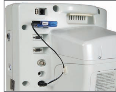
Criticare Connect shown attached to the nCompass™ vital signs monitor
