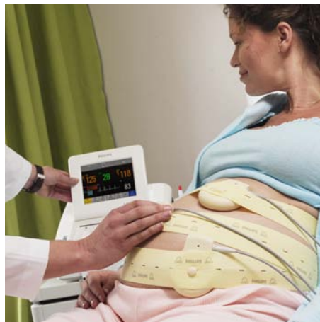
The Avalon FM20 and FM30 can monitor triplets with sophisticated three-channel ultrasound tracing capability and coincidence detection between all heart rate channels.
