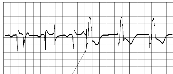
AVOID PACE PULSE REPOLARIZATION TAILS (NOTE WIDTH)
