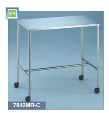
MODEL 7842MR INSTRUMENT TABLE. New and improved design offers complete 18-gauge, type 304 stainless-steel construction. Lightweight, yet extremely durable. Sanitary closed top hem prevents bacterial build-up. Sealed reinforcing channels provide structural rigidity. 1-1/4"-diameter legs are fully welded for strength and stability. H-braces are fully welded around the legs with no crevices for dirt to collect. All tables travel easily on two-inch, MR-Safe casters.
