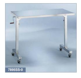
**ADJUSTABLE HEIGHT INSTRUMENT TABLES** offer twenty inches of travel to accommodate changes in OR table position during neuro, cardiac and orthopedic surgery. When used in general surgery, the table can be adjusted to accommodate the varying heights of personnel. This model can be adjusted manually from either side with a detachable crank handle. Tables travel easily on four, 3" casters, two casters with brakes.
